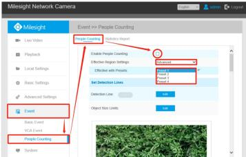
**Step 2:** Click *Edit* of *Detection Line* and draw a line. The direction of the arrow is IN. If necessary, you can also set Min and Max size limits of object to exclude abnormal targets.
